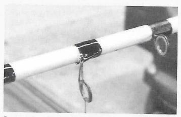
Test results showed that wraps where epoxy finish is applied directly to the threads to be only marginally stronger than those where color preserver was also used. Results are relative in nature and not an accurate indication of what all guide types, threads, color preservers and finishes will produce.
