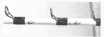
10 test sticks with 3 guides each were prepared. On each stick a guide was wrapped and coated with epoxy wrap finish only, color preserver only, and color preserver and epoxy wrap finish. Each specimen was then loaded at 90 degrees to the mount until the guide to blank bond was broken. (Remember that such a test must be judged upon relative strength of the wraps to each other and may not be indicative of the varied forces placed upon rod guides in actual use.)
