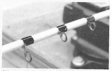
Guides used were single foot high-frame #12's. In each instance the guide frame seriously distorted before the guide to blank bond was broken.
