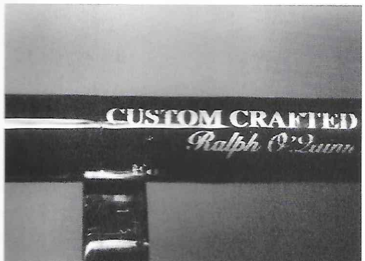
Using the straight ended spatula to apply epoxy resin to a long thread and inscription area. This is also done while the rod is turning.
