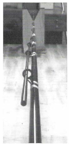
Here a spare fly rod blank tip section has been inserted through the first 5 guides of the Author's spiral guide placement system. Notice that it follows a very straight path, devoid of the sharp turns of most spiral wrap systems. The line will likewise follow this path and result in less friction and better casting qualities than in those systems where it must make sharp turns on its way to the underside of the rod.
