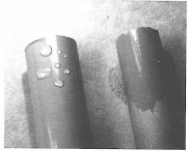
These photos illustrate the difference between the supplied surfaces of new rod blanks (left) and the surfaces of blanks which have been properly prepared (right) and are now considered in "water-break-free" condition.
